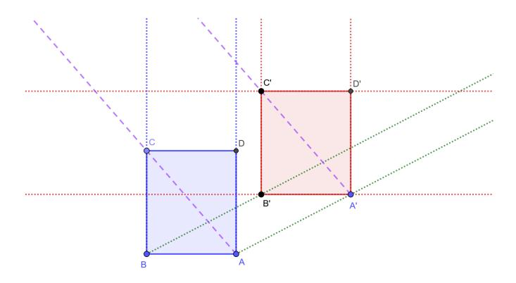
Notice that we can observe several sets of parallel lines. You are given the rectangle ABCD to start with, plus another point A'. You need to think of what sequence of constructions you would use to construct the points B', C', and D' (hint: I would probably construct them in that order). Use the fact that each set of parallel lines will have its own vanishing point on the horizon in perspective.
