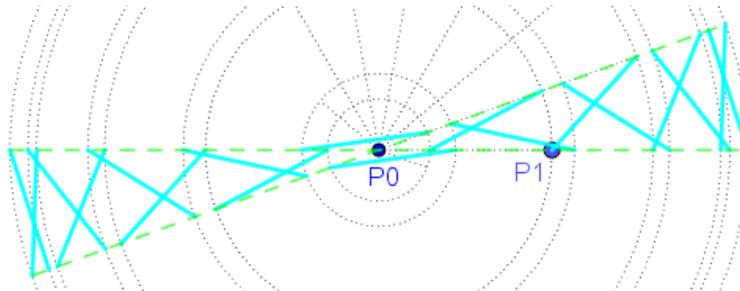
Now I trace the first circle with center in (P0) and with radius (R0), this circle intercepts (s0) in two points of which the one on the right for my choice is (P1) that is the point of both the basic and the polygonal pattern. From this point I trace the first blue segment with an angle ( $\alpha$ ) counterclockwise with respect to (s0) as in the previous example, the length of this segment I have already explained to be delimited by (s1).
