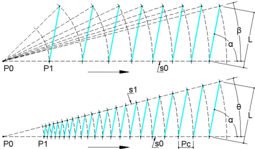
The purpose of the basic scheme is to define the length, inclination and mutual bond of the blue segments, the rotated copy of these segments then forms the polygonal.
